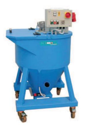
• The photo alongside shows a vertical mixer for mixing small quantities of product or, as is often the case, for moulding tests or materials test.
